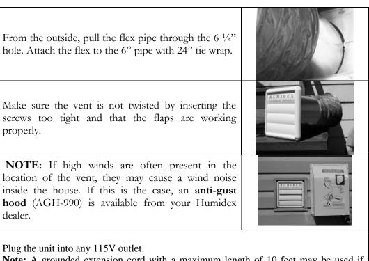
**Note:** A grounded extension cord with a maximum length of 10 feet may be used if necessary.
